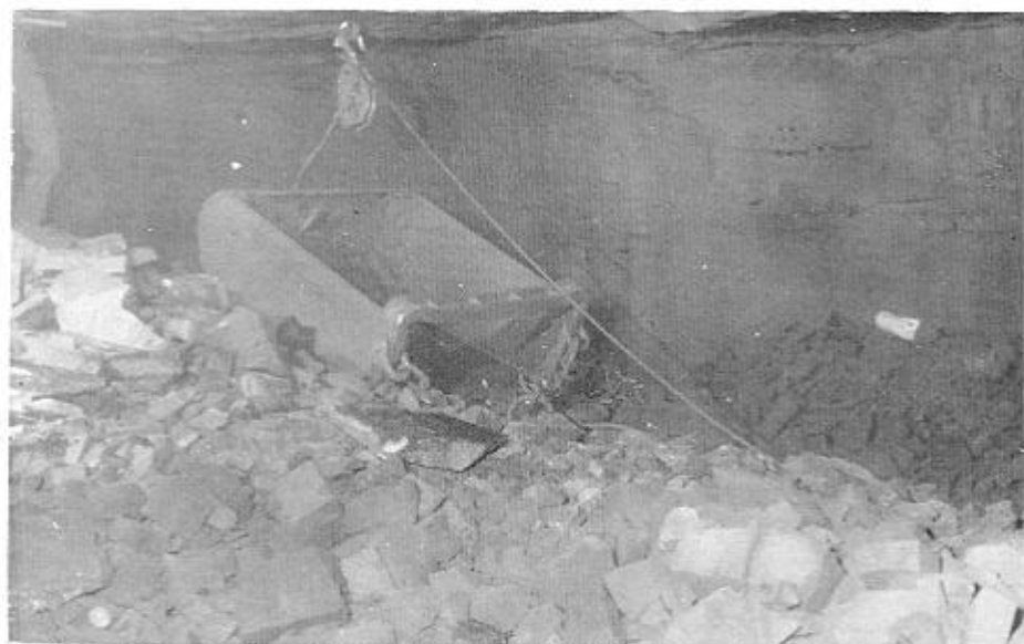
SLUSHER BUCKET BEING POSITIONED AT FACE. IMMEDIATELY ABOVE THE BUCKET CAN BE SEEN THE GYN BLOCK.
