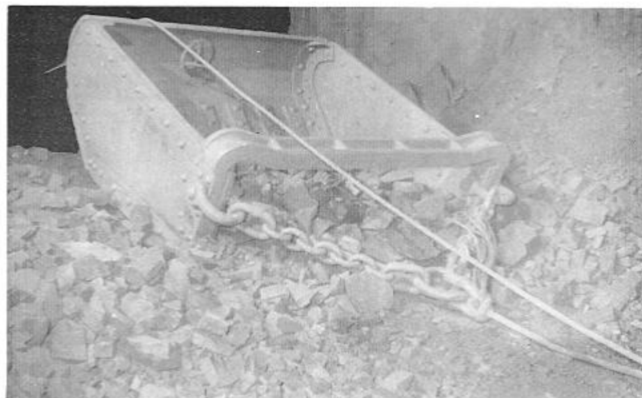
SLUSHER BUCKET GATHERING ORE ON WAY TO LOADING RAMP
